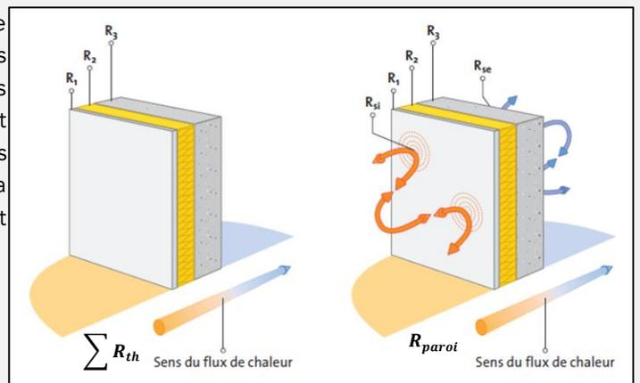
$$R_{paroi} = R_{si} + R_{se} + \sum R_{th}$$
